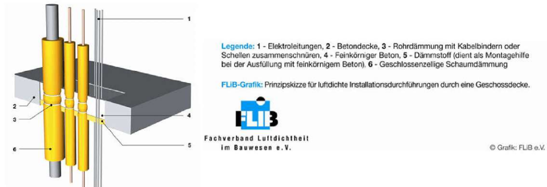
Figure 13. Insulation requirements for pipes (Building physicist 2017c)
