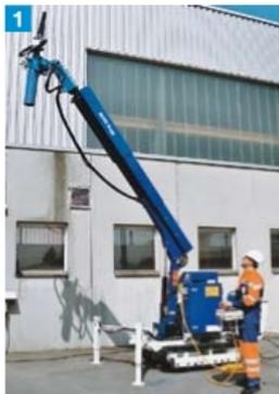
**1** The MEYCO Rama 4 spraying manipulator is compact yet has two extensions to allow great reach, powered by a 7.5 kW electro-hydraulic drive unit.
