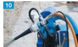
**10** Standard full size MEYCO spraying head for ideal spraying position and strength to enable use of dia. 65 mm or even 80 mm wet-spraying nozzle.
