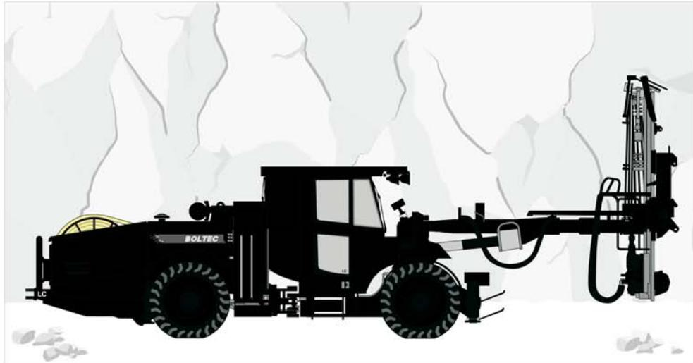
A fully mechanized rock bolting rig with RCS based control system for high productivity and precision. For bolt lengths 1.5–6 m and effective in roof heights up to 12 m.
