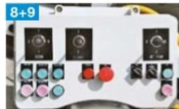
**8+9** Electric remote control with 15 m cable (or radio as option) controls all manipulator functions.
