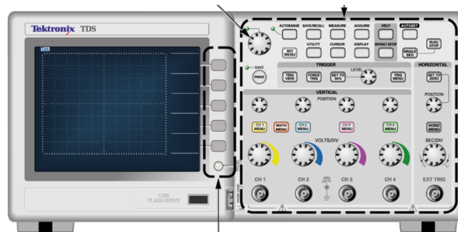
Figure A.2: 4-channel oscilloscope similar to the one used. (from the Tektronix manual: "TDS1000B and TDS2000B Series Digital Storage Oscilloscopes")
