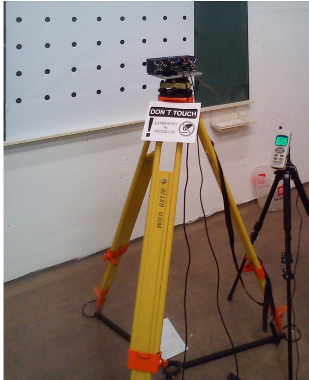
Figure 3.8: The final set up. Tripod with mounting plate on top around one meter away from the target pattern on the blackboard.
