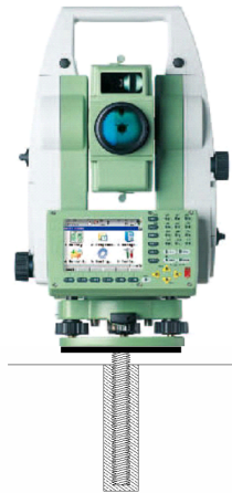
Figure 1.1.2: Mounting of the total station in the bedrock
