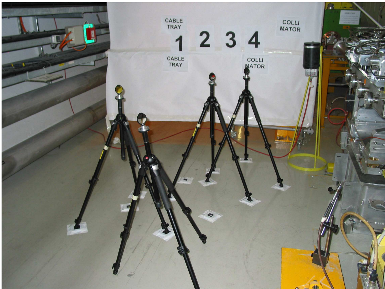
Figure 4.5: Picture of the fixed mirrors in front of the collimator (on the right side). In the back the paper wall for aiming the laser beam with the help of webcams onto the correct measurement point can be seen. One can see that the mirror for the measurement point #2 was not in line with those for measurements #1, #3 and #4. Wilfinger (Picture courtesy Roman Wilfinger [142])
