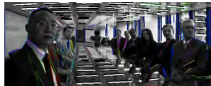
(b) Line detection and grouping using LSD [160] and J-Linkage [147]. Each line class is represented by a different color [46].
