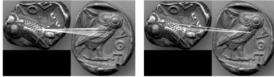
(a) single descriptor from the test image is matched against multiple descriptors from the training image, and ...
