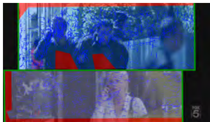
(d) Clusters that are not separated by a uniform area are merged. Red color: non uniform area. Green color: uniform area surrounding a motion cluster.
