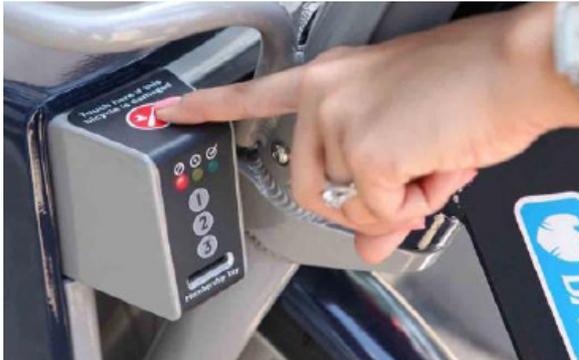
Figure 139: Device in the docking point used by customers to report damaged bicycles in the Barclays Cycle Hire of London (Georgiou 2010).
