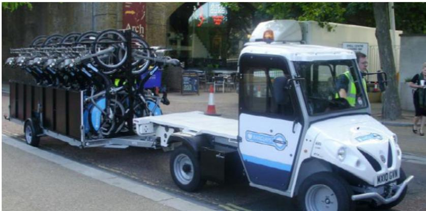
Figure 141: Electric vehicle for redistribution in Barclays Cycle Hire, London. Source (Georgiou 2010)
