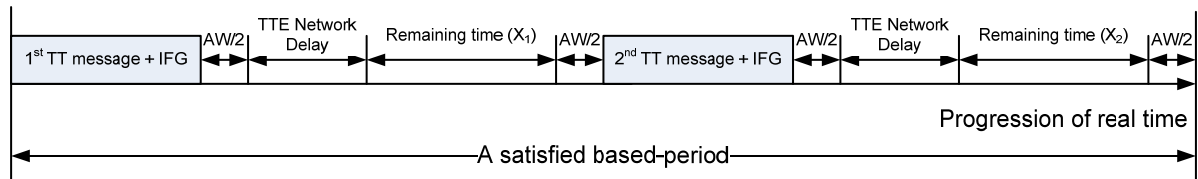
Fig. 5.15: Remaining times in distributed offset form in consideration of TTE network delays
