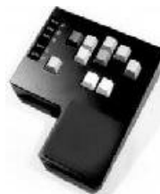
Figure 4.9: An approach of an adapted keyboard for people with disabilities in using both hands [66].
