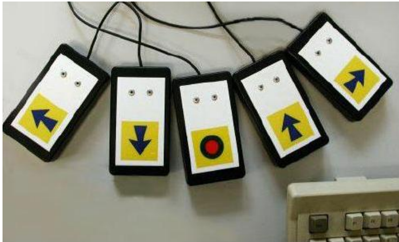
Figure 4.8: An approach to control a computer mouse for people suffering from cerebral palsy [66].
