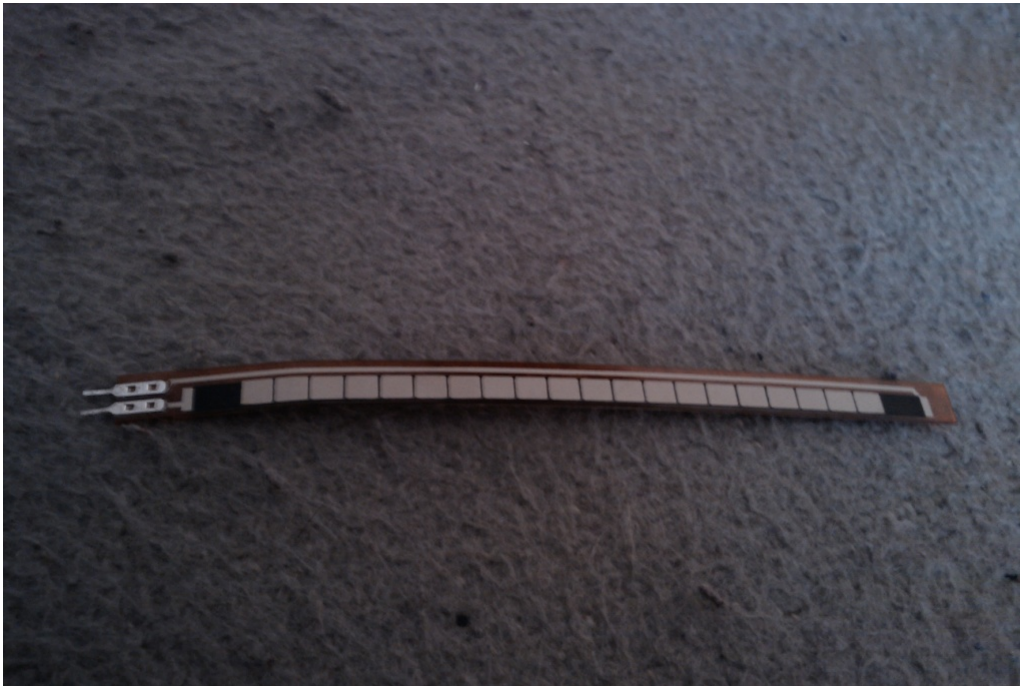
Figure 6.2: The Flex sensor manufactured by Spectrasymbol.
