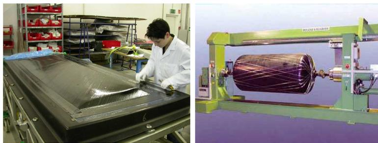
Figure 1.3: Manufacturing of laminated structures; hand lay-up of prepregs (left) courtesy of FACC AG, Ried, Austria; filament winding technology (right)[2].
