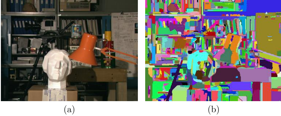
Figure 5.3: Colour segmentation. (a) Left image. (b) Computed colour segmentation.
