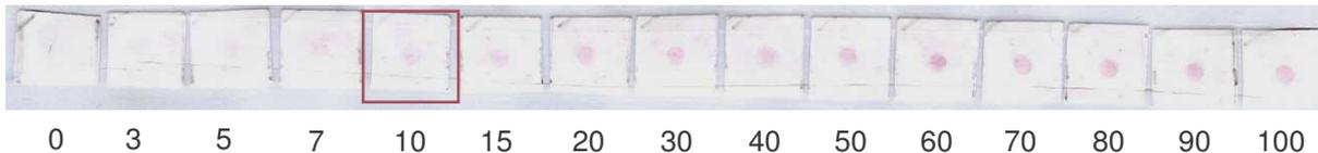
**Figure III.30:** Dipstick results detecting various hazelnut concentrations in  $\mu\text{g}$  nut/10ml
