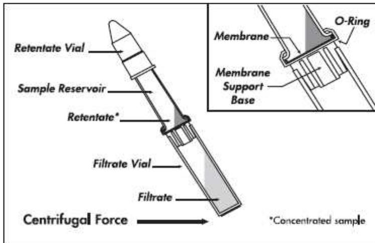
Figure II.20: Centricon Centrifugal Filter Device (© millipore)
