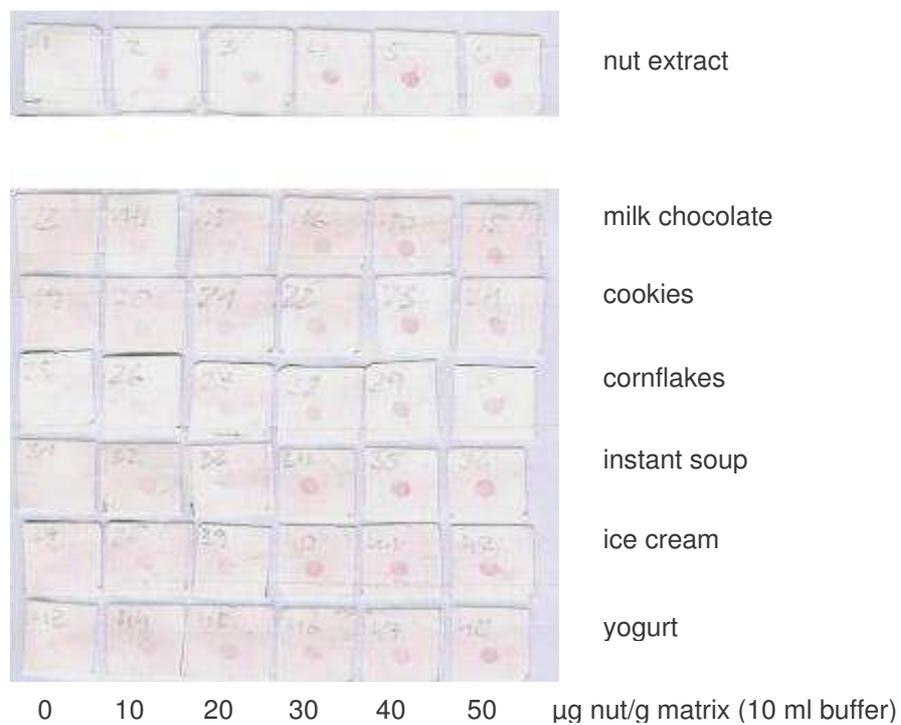
**Figure III.32:** Matrix samples on hazelnut dipstick
