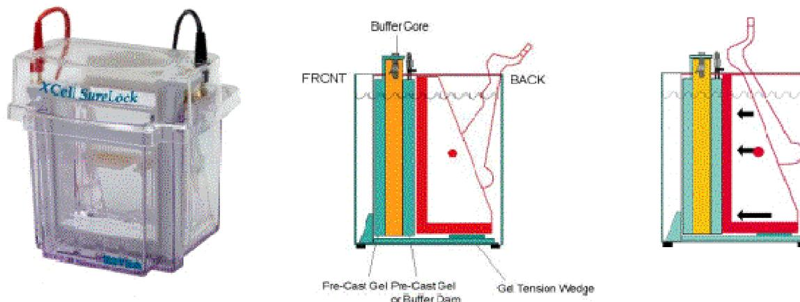
**Figure II.19:** Schema of the XCell SureLock™ Mini-Cell electrophoresis unit (© invitrogen)
