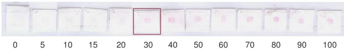
**Figure III.29:** Dipstick results detecting various peanut concentrations in  $\mu\text{g}$  nut/10ml
