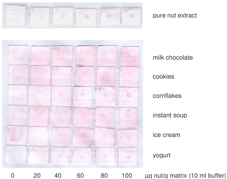
**Figure III.31:** Matrix samples on peanut dipstick
