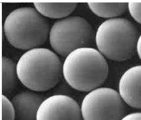
**Figure I.8:** Scanning Electron Microscopy image of polystyrene microspheres
