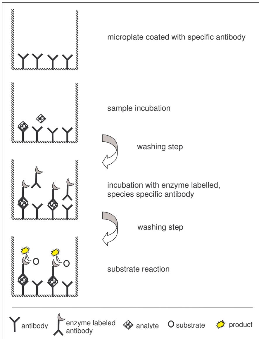
Figure I.12: Principle of a sandwich ELISA
