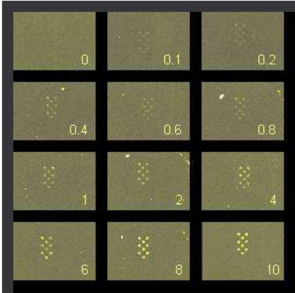
**Figure III.36.A:** Scan of observed fluorescence signals for peanut samples [ $\mu\text{g}$  peanut/ 10 ml]
