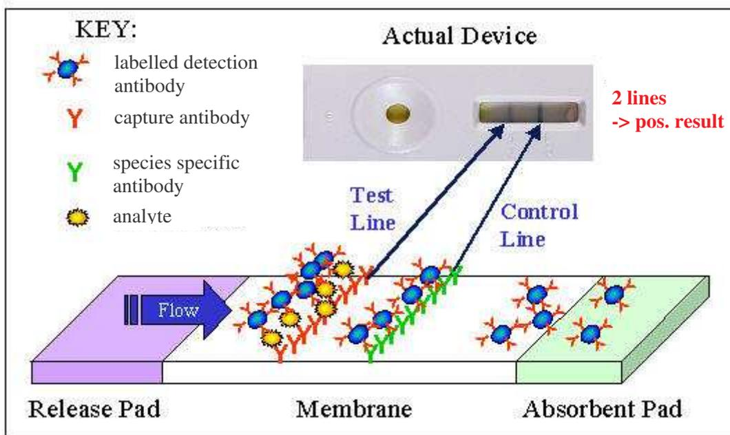
Figure I.13: Principle of a sandwich LFD (© by Chris Danks, CSL, U.K.)
