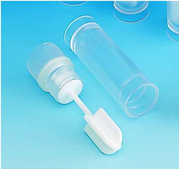
**Figure I.15:** Example of an immunostick paddle [Canadawide Scientific]
