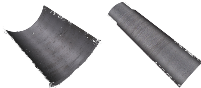
Figure 9: Real 3D-images of an exemplary worn bearing (left) and matching shaft (right) surface measured with the Alicona 3D-microscope.
