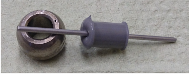
Figure 8: Worn porous bearing and silicone replica of its inner bearing surface. Note the 0.6 mm hole for the thermo-couple in the front face of the bearing.
