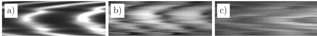
Figure 18: FECO data from different SFA-runs; a) control run against flat Au in transmission mode (FECO=white), b) better quality data (FECO=black), c) poor quality (FECO=black).
