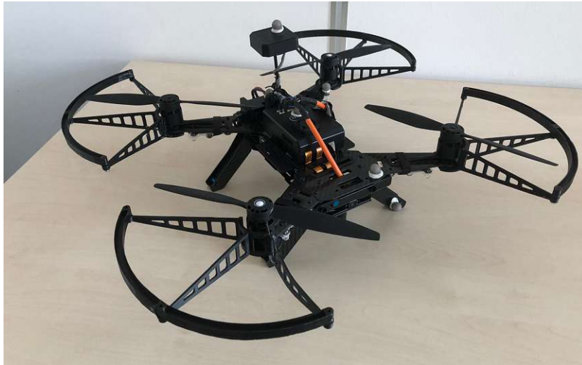
Figure 3.1: Intel Aero ready-to-fly (RTF) used in the thesis [35].
