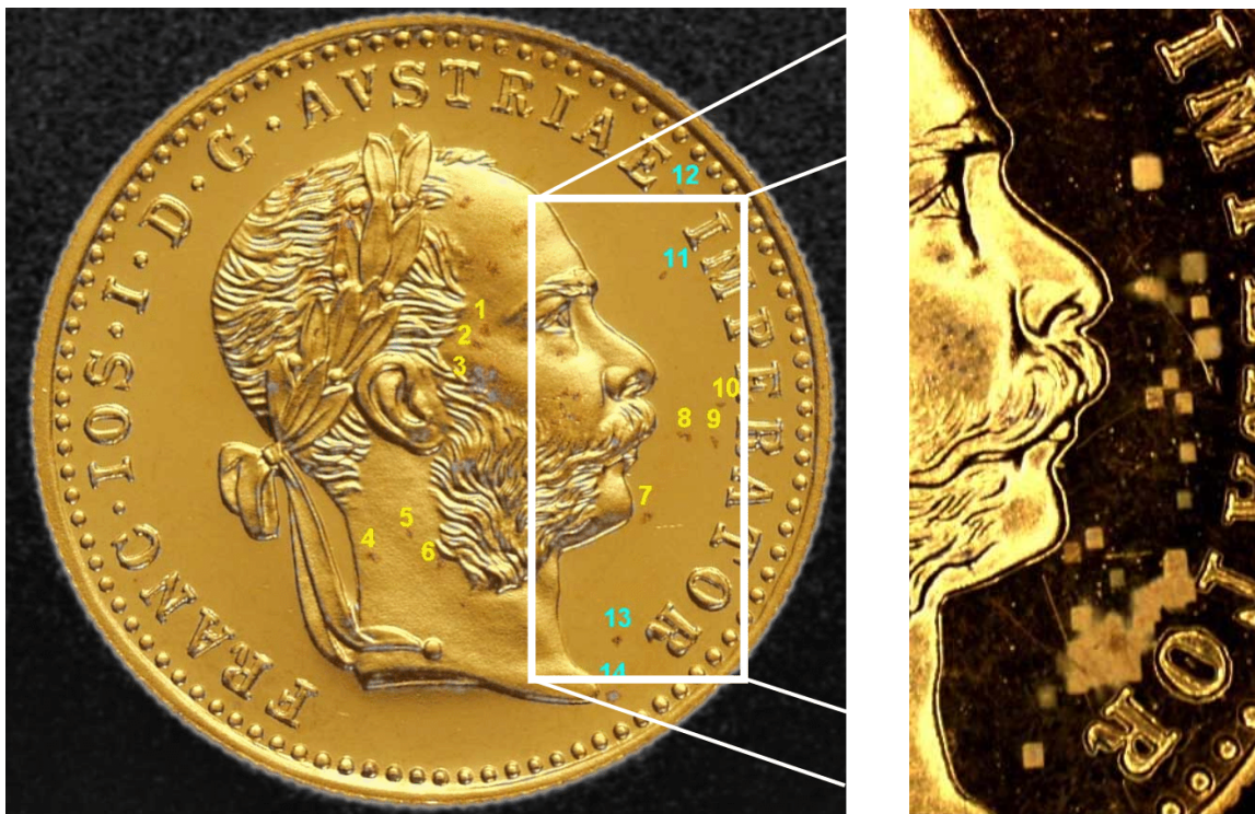
Figure 44: left side: front side of ducat Ag before SIMS measurements; suitable sites for SIMS investigations are labelled;
