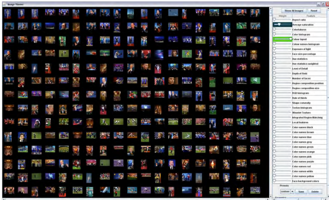
Figure 1.4: Screenshot of the APA demonstrator. Example journalists' search for images with red carpet on the bottom and blue background: The query image is a reasonably satisfying image (upper left). The journalist chooses to retrieve images with close color layout and similar average saturation.
