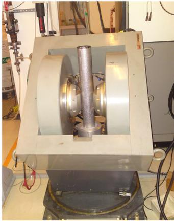
(a) View on the rotating magnet and the cryostat.
