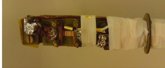
(b) Mounted sample on the single axis sample holder.
