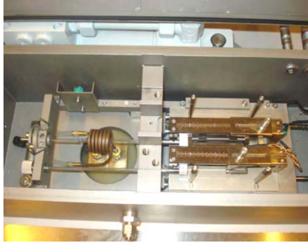
Figure 4.7: Chamber containing heating, cooling and dilatation measurement system.
