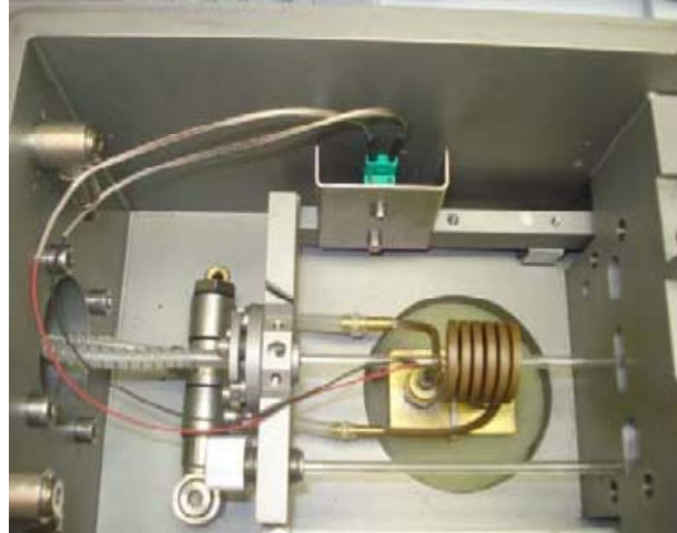
Figure 4.10: S-type (Pt/Rh 10%-Pt) thermocouple attachment with the dilatometer and sample.
