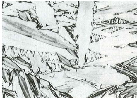
Figure 3.16: Plate martensite in high carbon steel [22].
