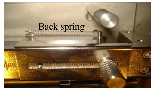
Figure 4.15: Back spring of LVDT.
