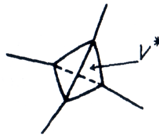
Figure 3.41: Critical nucleus shape for nucleation on a grain corner [6].
