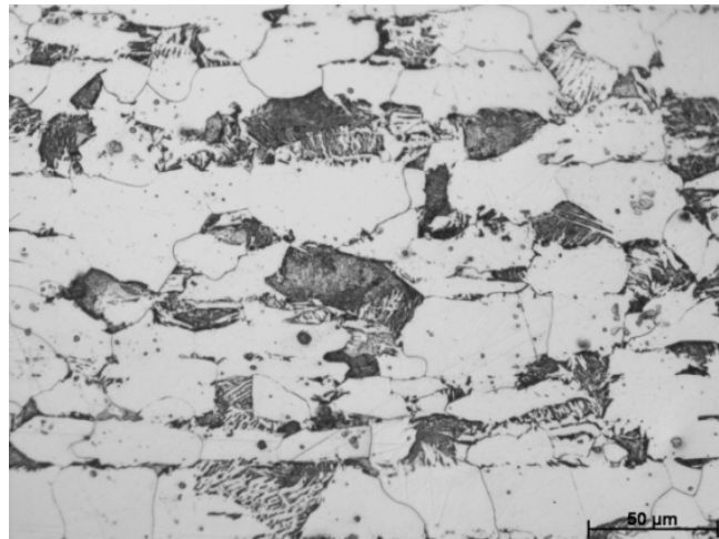
Figure 6.24: Microstructure of alloy D obtained at a target IT temperature of 760°C, showing mainly ferrite with pearlite islands.
