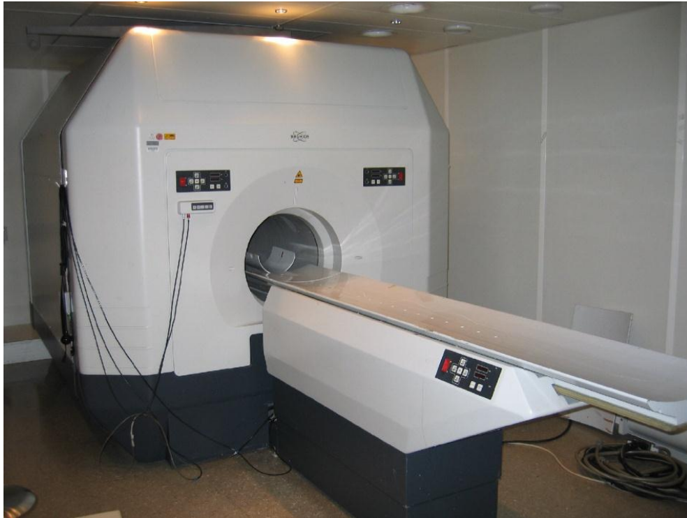
Figure 30: 3 Tesla Bruker MedSpec S300 whole-body scanner The scanner is located at the MR Center of Excellence in Vienna
