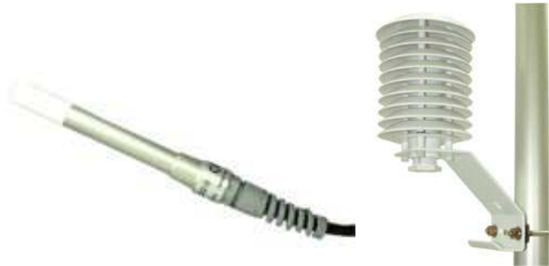
Pic. 6 Combined CS215 Temperature and Humidity Probe (left) and a radiation shield 41303-5A (right)
