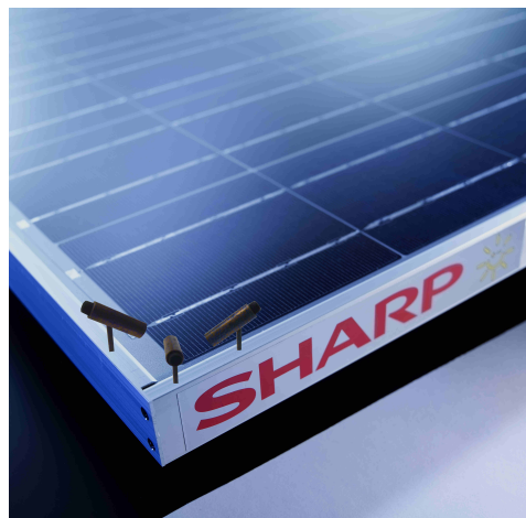
Figure 28: Module with pollution detection sensor
