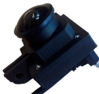
Figure 4. Low-cost IDS camera UI-3251LE-M-GL, resolution: 1600 by 1200 pixels at 60 Hz.
