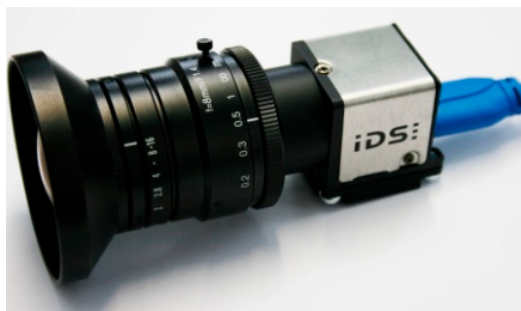
Figure 3. IDS camera UI337, resolution: 1024 by 1024 pixels at 100 Hz.
