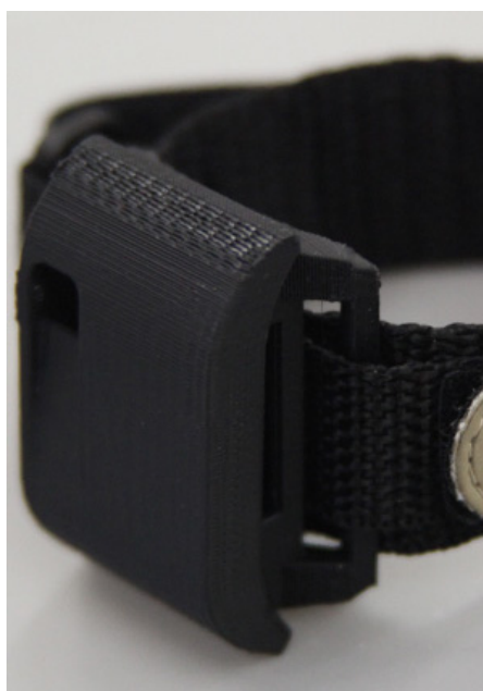
Figure 2.4: The self-care technology by McNaney et al. (2011), here named Cueing Swallowing , is a wearable device that produces a vibration cue every minute. Its goal was to alert patients of the need to swallow the saliva excess. The figure shows a picture of the device (Credits: http://openlab.ncl.ac.uk/v2/wp-content/uploads/2010/08/PDQ.jpg by Open Lab).
