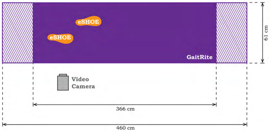
Figure 5.14: The setup for the validation measurements inside the social medical center Sophienspital. The upper half shows one patient walking over the GAITRite ® mat, while wearing a pair of eSHOE insoles. For synchronization of both systems a video of the patient's feet was recorded with a camera mounted onto a self-made cart. The lower half shows a schematic diagram of the measurement setup. The version of GAITRite ® which was used in this study measured 460 \times 61 \text{ cm} , with an active sensor area of 366 \times 61 \text{ cm} . The part of the walkway without sensors is indicated by the shaded sections.
