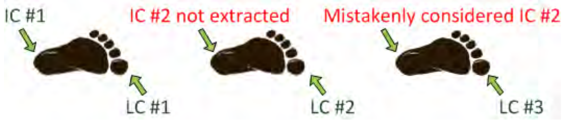
Figure 5.13: initial contact (IC) extraction error. Visualization of extracted gait features in left insole data where one IC could not be extracted by the algorithm. Adopted from [Reich, 2013].
