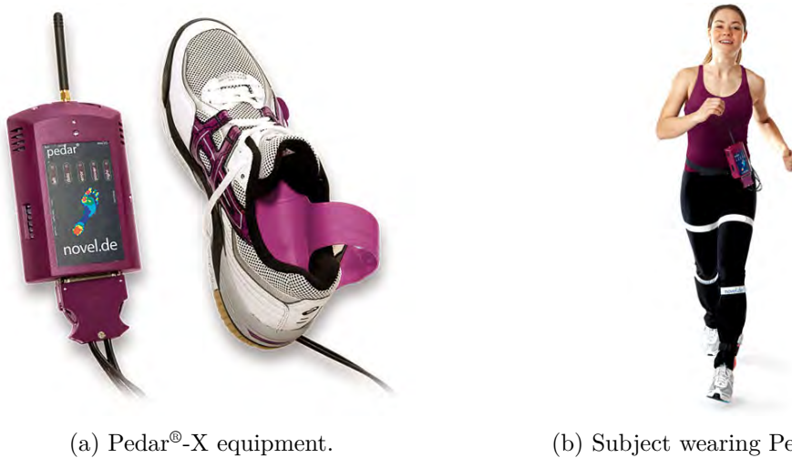
Figure 3.6: Pedar ® -X insole pressure measurement system. (a) retrieved from http://novelusa.com/index.php?fuseaction=systems.pedar , viewed 01.09.2016; (b) retrieved from http://novel.de/novelcontent/pedar , viewed 01.09.2016
