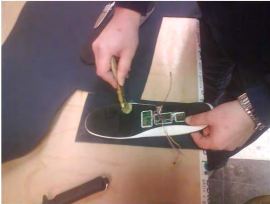
Figure 4.10: This picture was taken during the manufacturing process of eSHOE prototype II. It shows (the hands of) an orthopedic technician, applying glue on the top half of an insole. This represents the last step in the manufacturing process.
