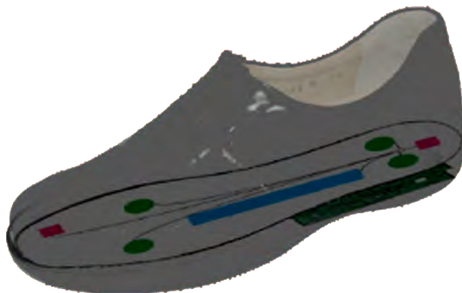
Figure 4.2: Conceptual schematic of the original idea for eSHOE.
