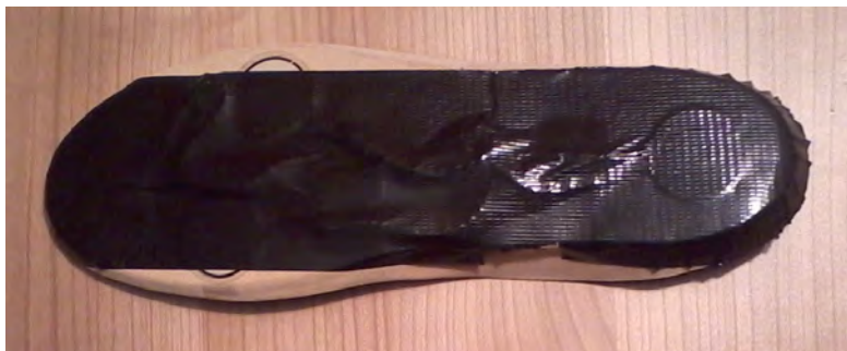
Figure 4.25: Final stage of the eSHOE insoles in the manufacturing process. FSR sensors and free wires are now covered with gaffer tape for (their) protection.
