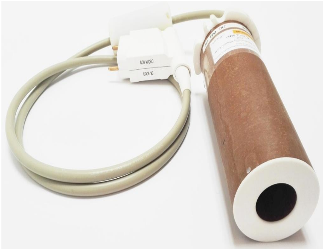
Figure 39: Complete view of the 8 channel receive-only coil.
