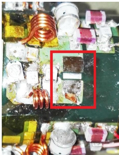
Figure 36: Removing the solder pad from the PCB.
