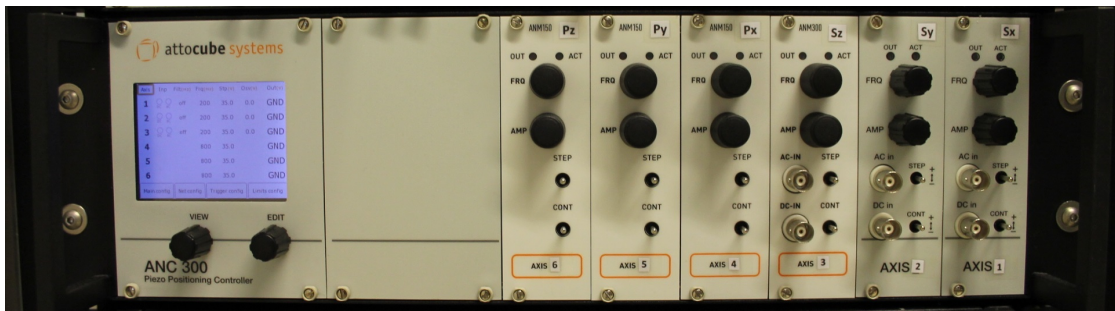
Figure 2.4: ANC300 with six modules, three ANM150 and three ANM300. From left to right, these are the coarse z-, y- and x-axes (labeled with “Pz”, “Py” and “Px” for “positioning”) and then the fine z-, y- and x-axes (labeled with “Sz”, “Sy” and “Sx” for “scanning”).
