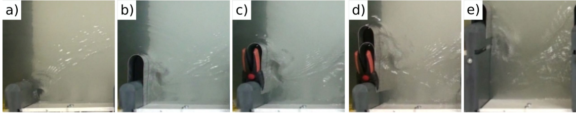
FIGURE 4.31: Vortex appearance at the third gate during test series B3; location of vortices at: a) l_p/b = 0.28 , b) 0.58, c) 0.71, d) 0.92 and e) 1.13
