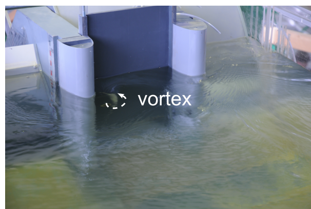
FIGURE 3.2: Vortex in front of the planar sluice gate during pre tests
