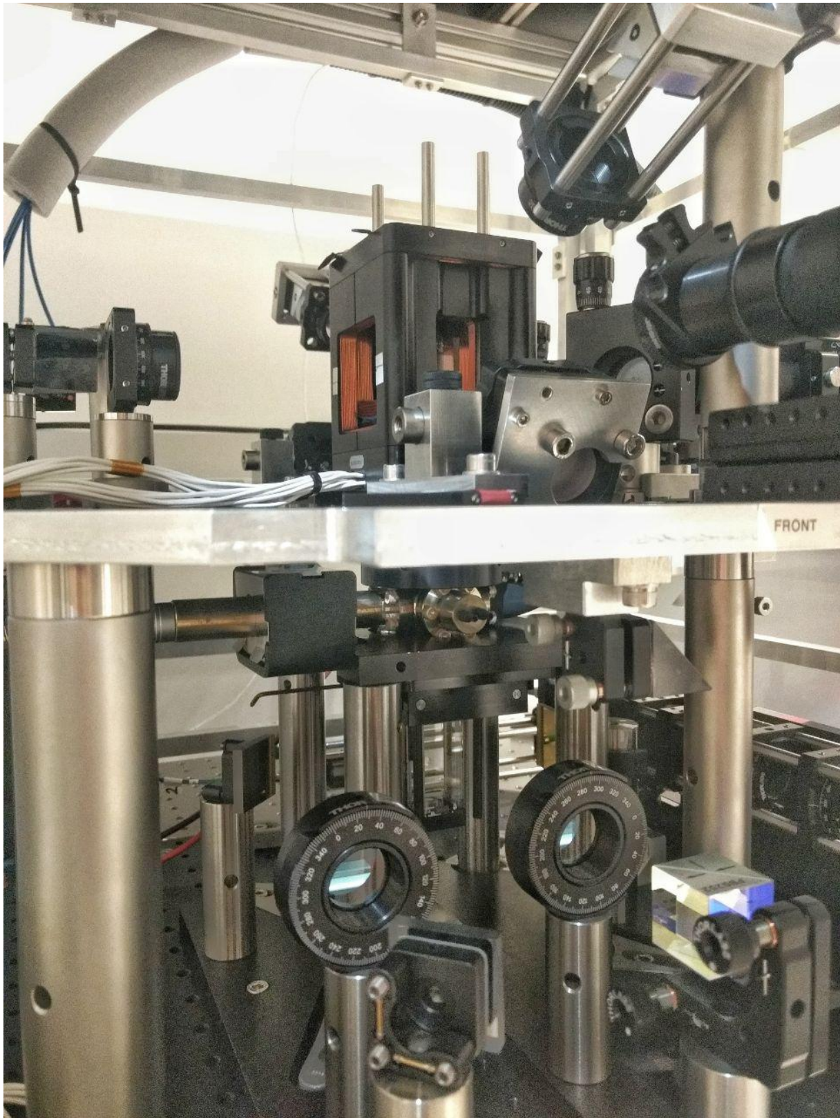
Figure 5.1: Photo of the Experiment. In the lower half you can see the PBS for the 2D MOT, the two \lambda/4 plates used for adjusting the polarization and the lower part of the glass chamber surrounded by the magnetic rods. Also the ion pump attached to the middle of the glass chamber. In the second half of the photo the coils surrounding the upper half of the glass chamber are visible.
