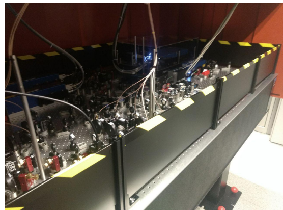
Figure 3.8: Pictures of the box protecting the dipole setup and the railing for the big laser table
