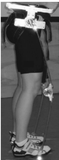
Figure 22: Unpowered exoskeleton design from Grabowski and Herr (2009).
