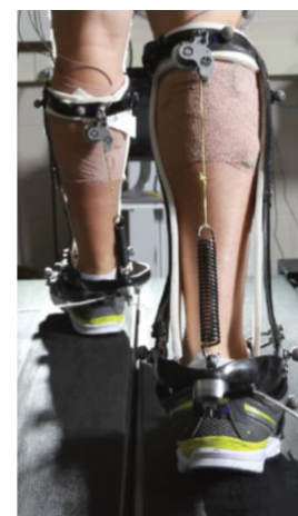
Figure 23: Unpowered exoskeleton design from Collins et al. (2015).
