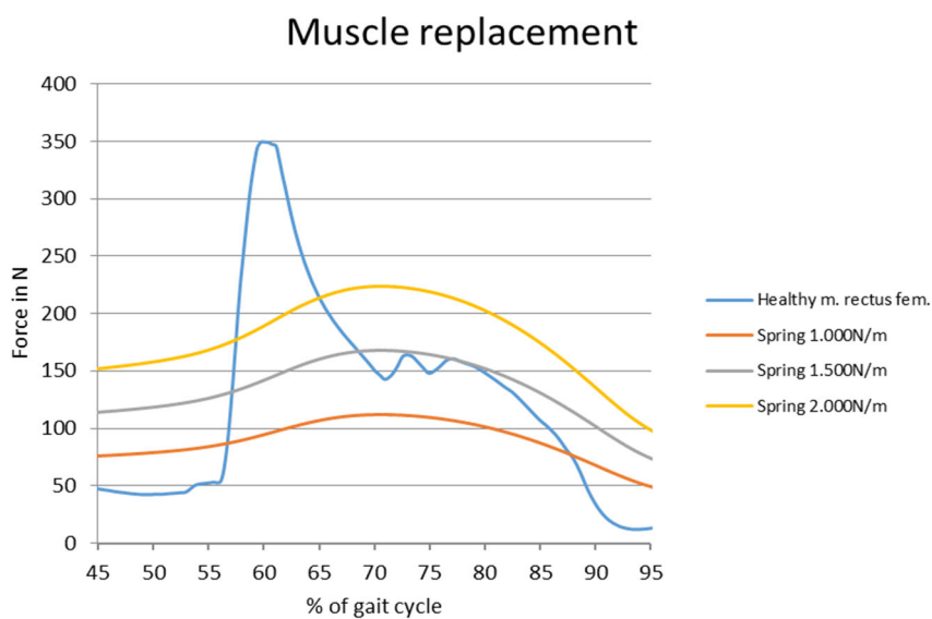
Figure 26: Replacement of m. rectus femoris by a path spring.
