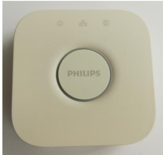
**Abb.20 Smart-Home-Basissystem Philips HUE Bridge**
