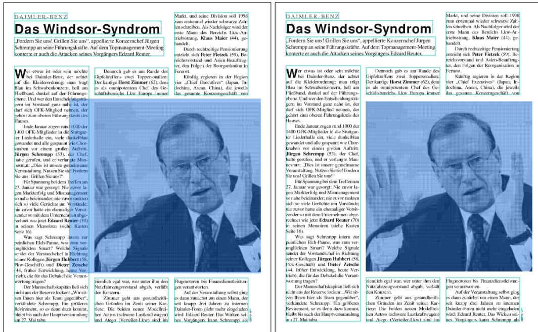
Figure 3.8: Page display without clipping (left) and with clipping (right) of an image
