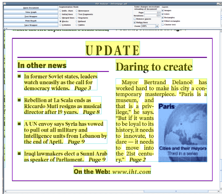
Figure 3.1: Screenshot of the GUI (see Section 3.2) showing some of these objects on the page. Line segments are marked in purple, image segments in blue. Clusters are shown in a cyan outline and their constituent text fragments are shaded in yellow
