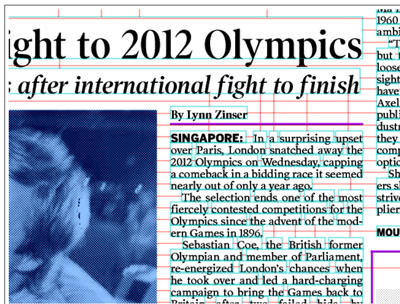
Figure 3.2: Example of a many-to-one adjacency relationship between the image and lines of text. Please note that the blue blocks represent the clusters at the initial stage of the segmentation process, before they have been merged together into larger blocks
