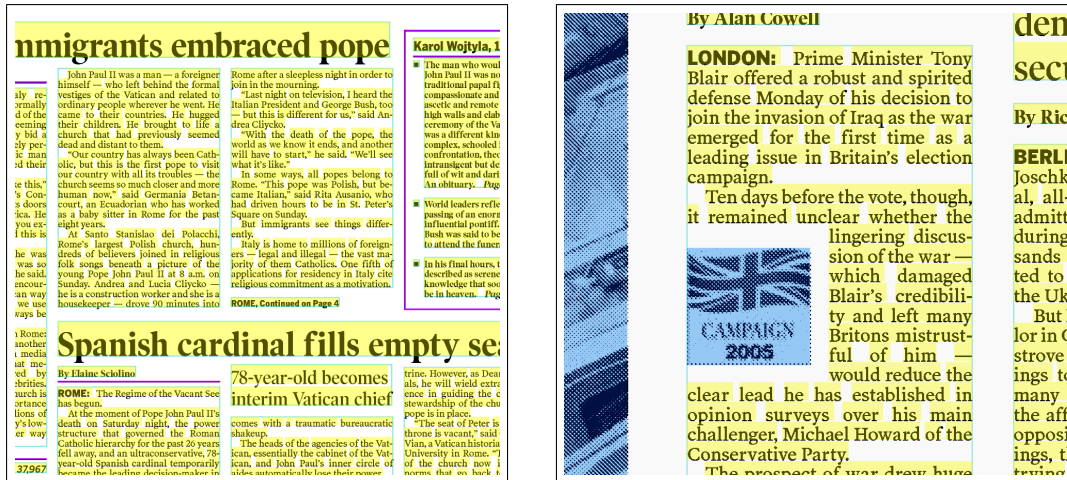
Figure 2.5: The example on the left has a strict Manhattan layout. The layout on the right is what we term near-Manhattan : because of the inset graphic, the conditions for strict Manhattan layout have been breached, but bottom-up segmentation can still be performed
