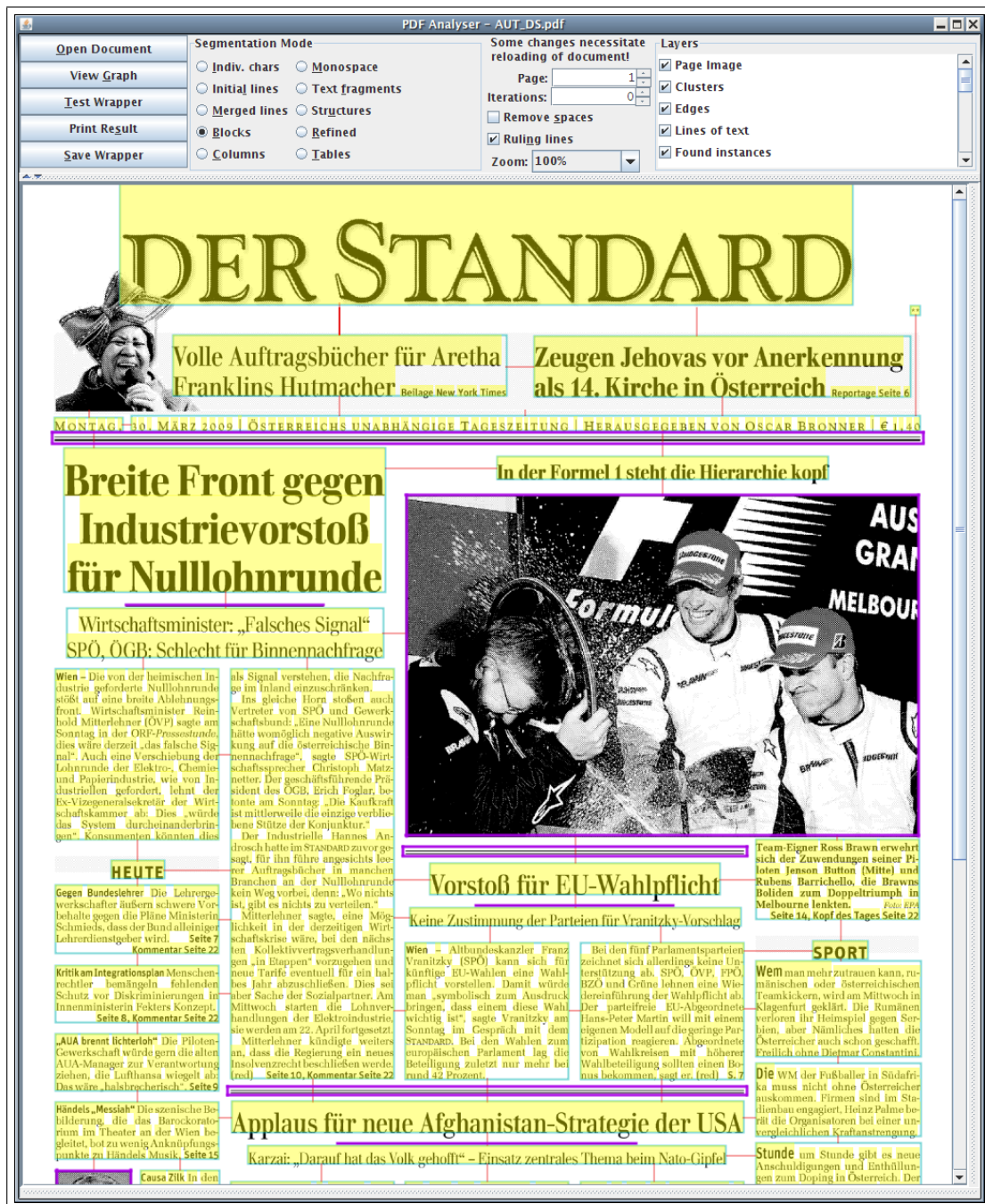
Figure 3.3: A further example of PDF Analyser's page view, based on methods in the XMillum library, showing the results of our segmentation algorithm overlaid on a bitmap rendition of the page. Adjacency edges between clusters are also shown here
