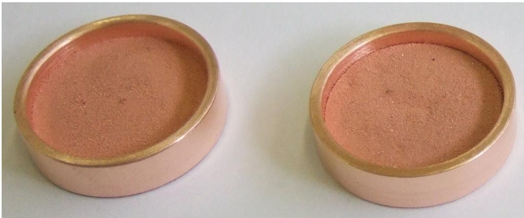
**Figure 5.8:** The sintered samples of the ESPI copper powder.
