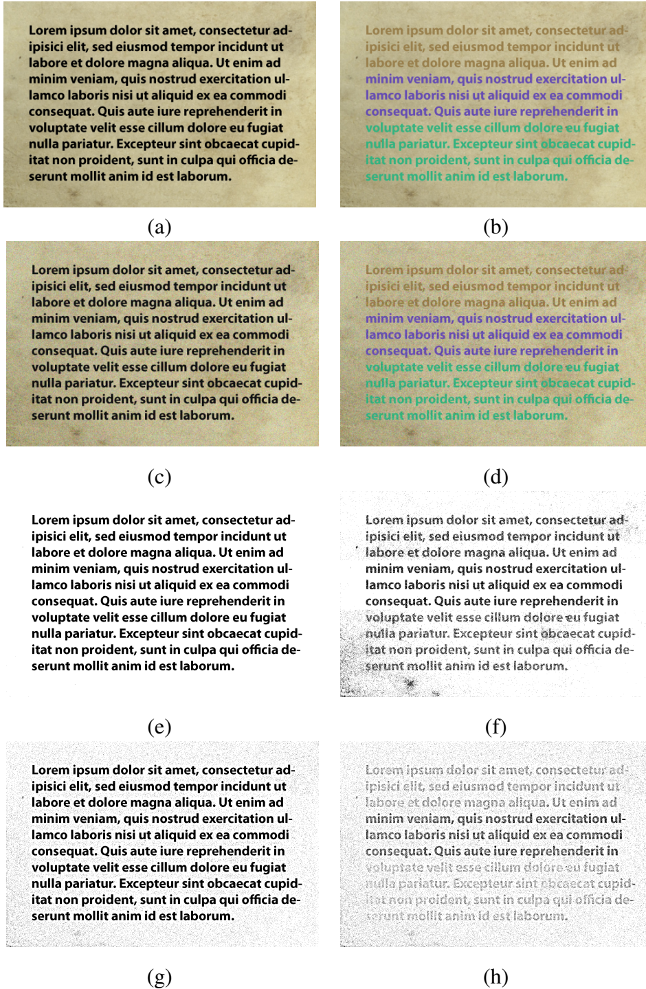
Figure 7.21: Synthetic image with black text in (a) and varying text color in (b). An image with Gaussian noise ( \sigma = 0.03 ) added is given in (c) for the image with black text, and in (d) for the image with varying text color. Results from the noisy image with \sigma = 0.03 are given in (e) and (f) for the proposed BP 5 algorithm, and for AB in (g) and (h). It can be seen that the proposed method has less noise in the background and foreground in both images, the image with black text and the image with varying text color.
