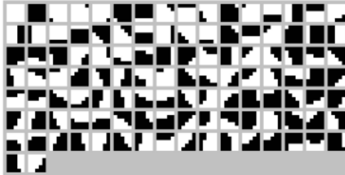
Figure 4.5: Examples for learning a prior model by means of image patches. The image patches are trained from high-quality binarized handwriting images. Therefore, the images are subdivided into 5 \times 5 image patches and the most representatives are learned by clustering. The remaining 114 patches serve as the hidden nodes for the binarization of handwritten reports, from (Cao & Govindaraju 2009).
