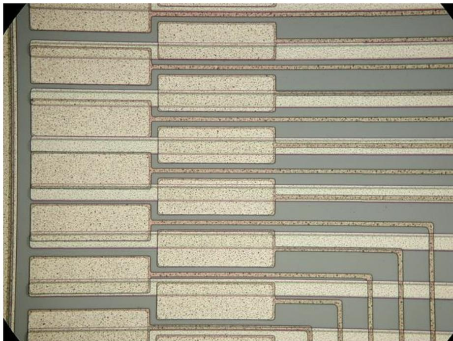
**Figure 9.22.:** Close-up of the contact pad region of a **Sensor2MPA** sensor. The location of each pad with respect to the strips depends on the strip number. Picture was made using a reflected-light microscope.
