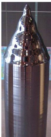
**Figure 3.8.:** A single crystal silicon ingot or boule.
