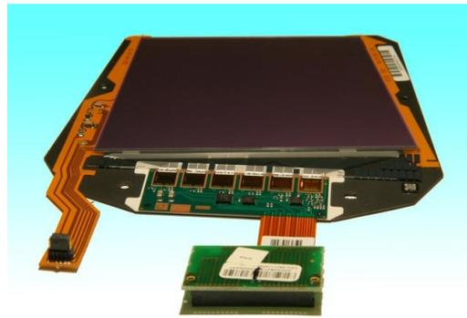
**Figure 4.4.:** Picture of a completed ring 2 module of the tracker endcaps.
