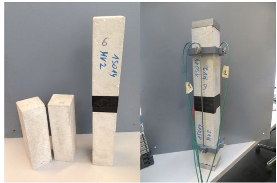
Fig. 2 Plain concrete prisms used for material testing: test specimens consist of two prisms in serial arrangement
