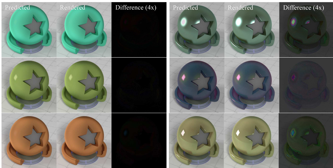
Figure 3.7: The best (left side) and worst-case (right side) predictions by our neural network on a set of 250 images. Mean PSNR: 37.96dB, minimum: 26.05dB, maximum: 48.70dB.
