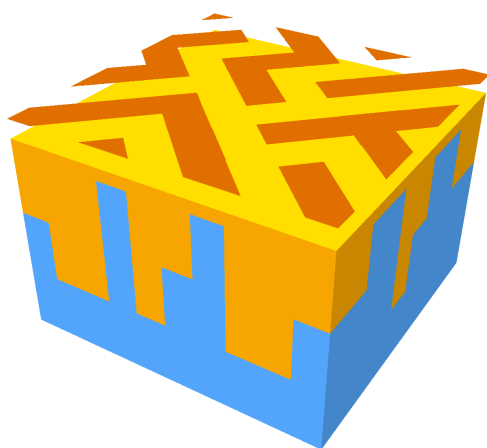
(a) The mask (brown) defines the pattern which is finally transferred onto the initial structure (blue) by partially removing the resist (yellow).
