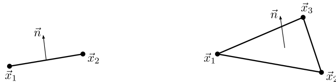
Figure 4.1: The orientation of the normal vector \vec{n} on a line segment and on a triangle as defined in this work with respect to the order of nodes \vec{x}_i .
