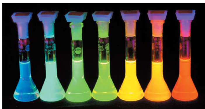
Figure 1.1. Size-dependent change of emission of colloidal suspensions of 1.7–5 nm core CdSe/ZnS core-shell NPs. Figure taken from Ref. 1.
