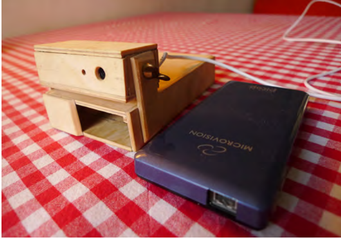
Figure 33: Pico projector and custom housing with IR camera.
