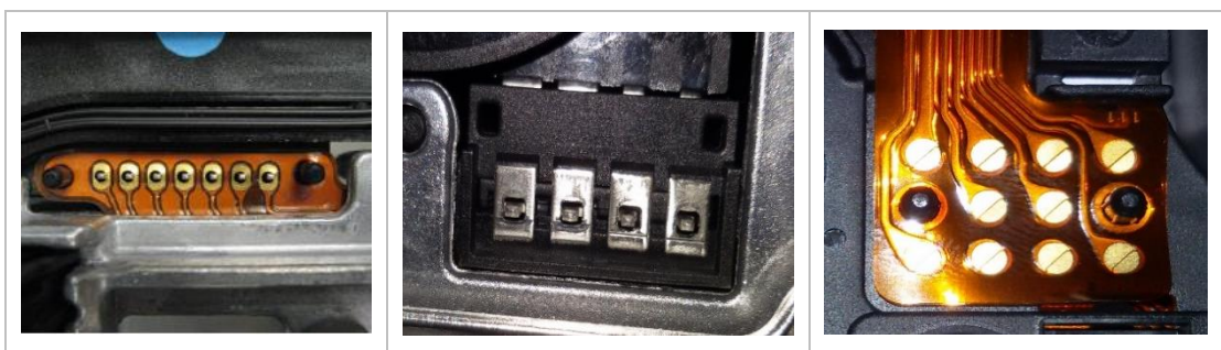
Figure 16: Types of soldering: Left – foil&pin; Center – metal&metal; Right - foil&foil
