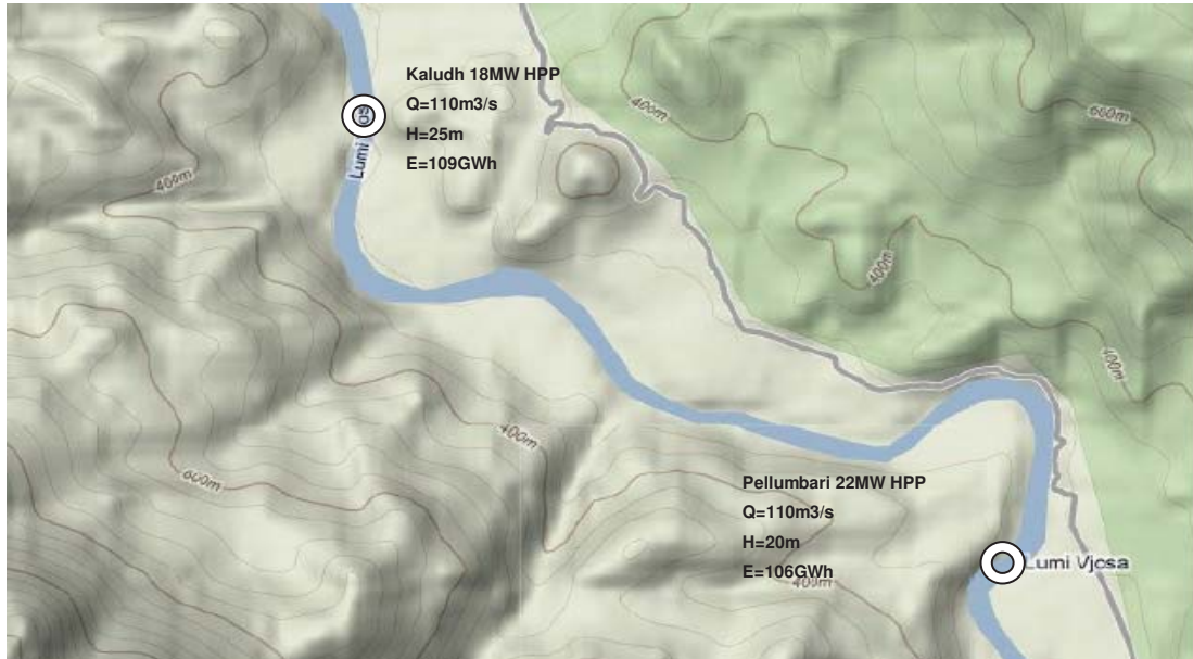
Figure A.10.11.1- Pellumbari 22MW and Kaludh 18MW HPPs
