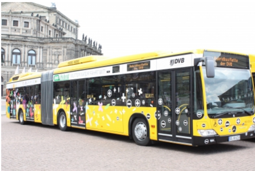
Figure 29: Serial hybrid bus on duty in the City of Dresden 100
