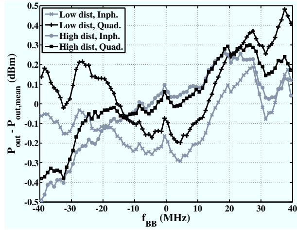
Figure 5.1: Relative output power of the inphase and the quadrature channel at the two operation modes.
