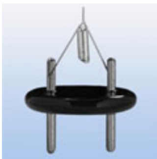
Figure 1.2: The bismuth liquid metal ion gun.
