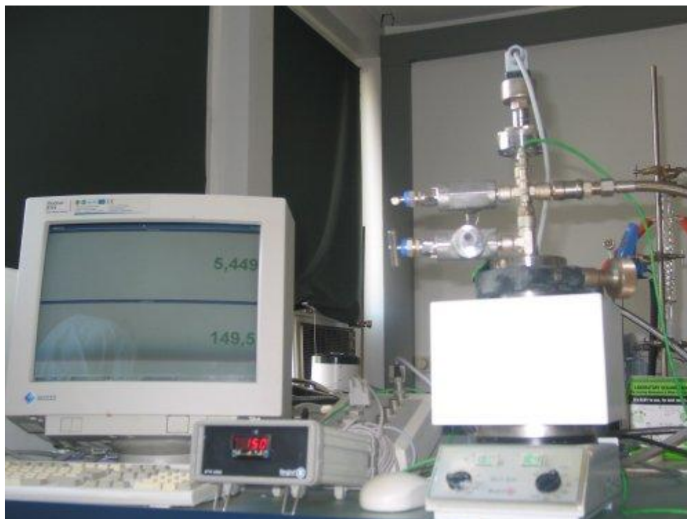
Figure 3-2 Autoclave BLH800 from Berghof- Germany, operated by computer using P4 MESS software to log temperature and pressure.
