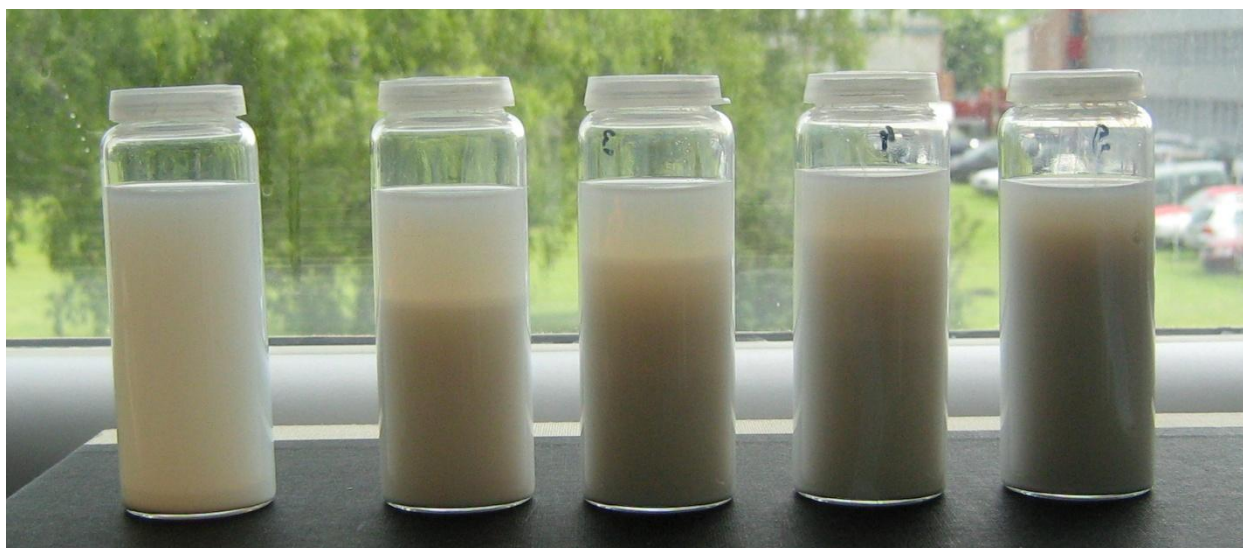
Figure 4-33 BaTiO 3 settling after 1h with Brij HLB variation for BaTiO 3 dispersion in THF, samples 5, 1, 3, 4, and 2 are shown in the figure for details of samples please see Table 4-VIII
