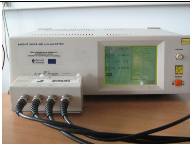
Room temperature condition and LCR meter used for capacitance measurements
