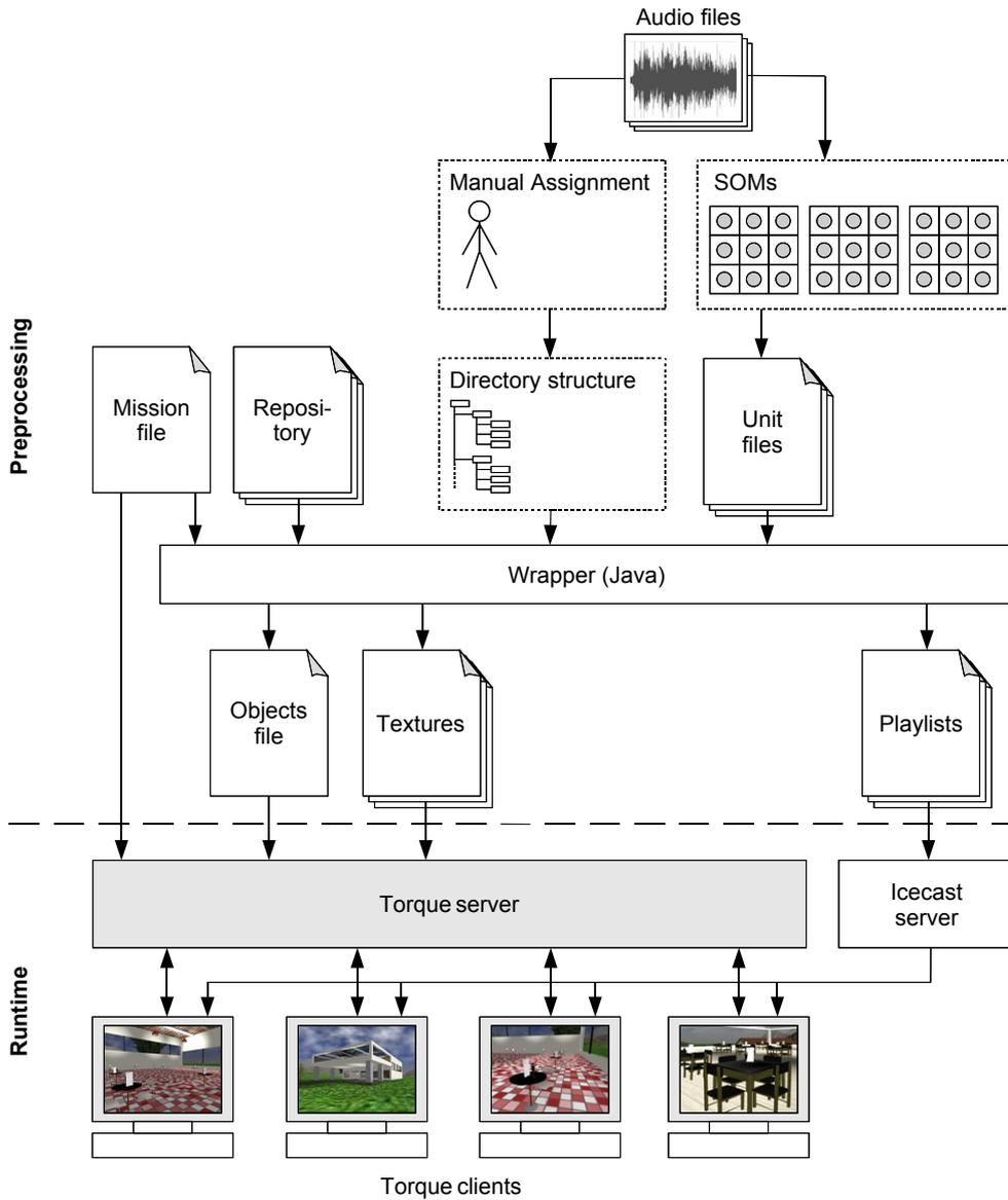
Figure 5.1: System architecture.
