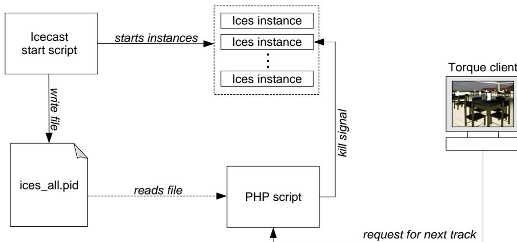
Figure 5.7: Setup for skipping tracks
