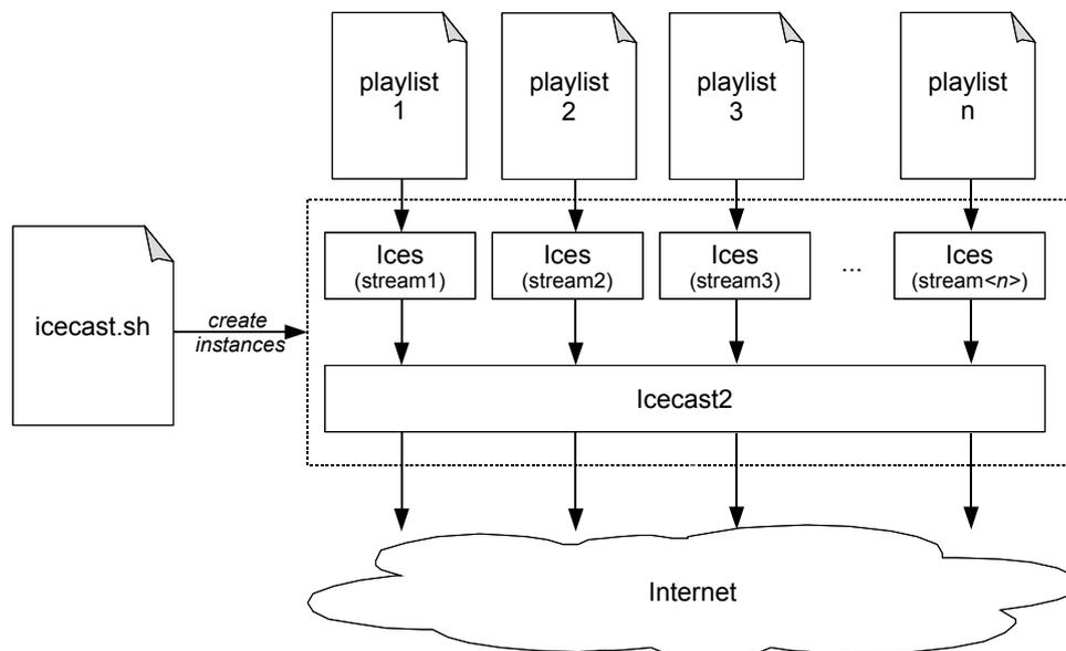
Figure 5.6: Icecast architecture
