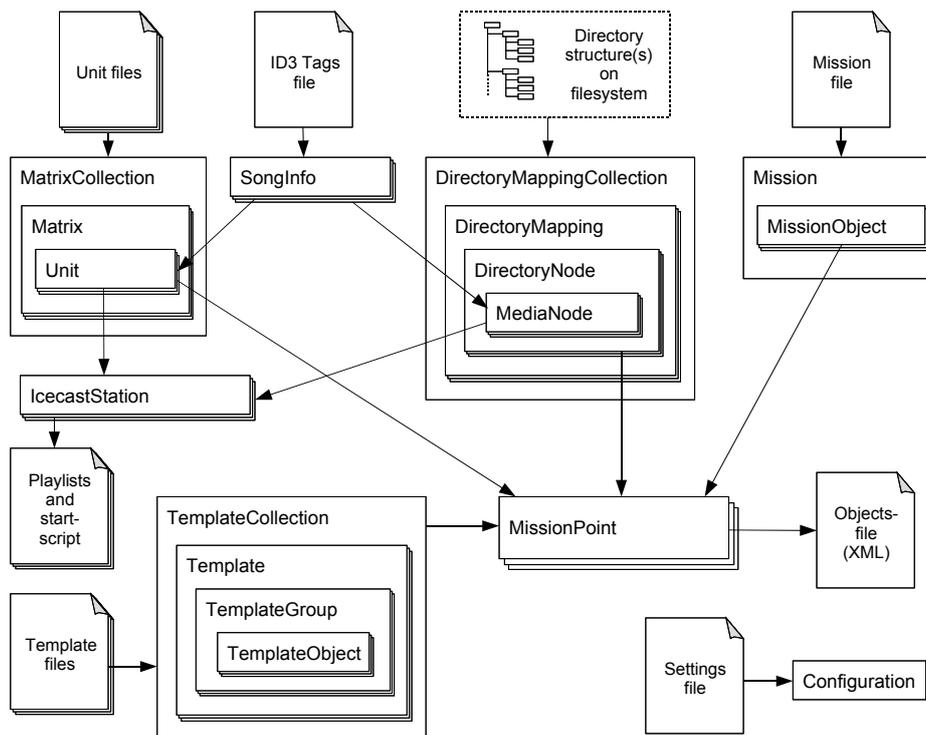
Figure 5.5: The Java-classes of the *Wrapper* support the representation and processing of the *mission-file*, one or more *unit-files*, one or more manually created directory structures, song-metadata, locations in the virtual environment and the *Icecast*-streams.
