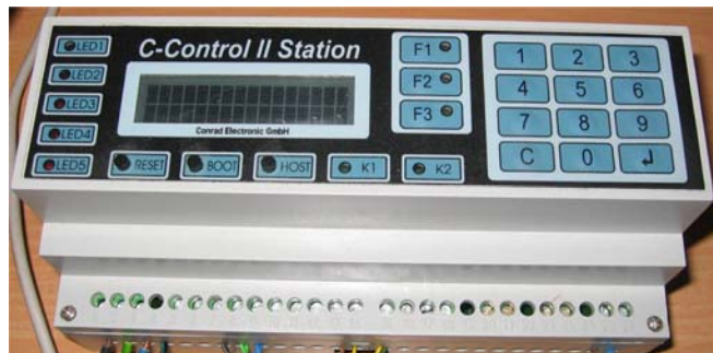
Abbildung 9-1: C-Control II Station
