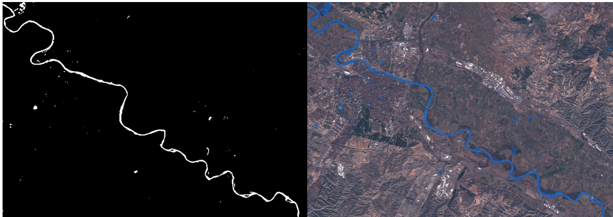
(a) Binary water map (white = water, black = non-water) (b) Water map polygon (overlying S-2 true-colour image from same date)
