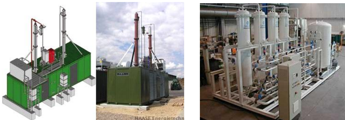
Figure 15: Biogas upgrading systems, water absorption system: source: Haase 2007, pressure swing adsorption system: Carbotec, 2007
